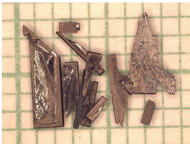
Figure 2.5 Fractionated melt flux grown, NaOH etched \text{AlMn}_2\text{B}_2 crystals
